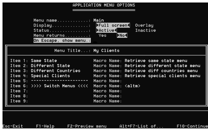
Figure 1. The "Switch Menus" selection (somewhat adorned) on the My Clients main menu with its corresponding Alt-M macro. The other "macros" are submenu names.
