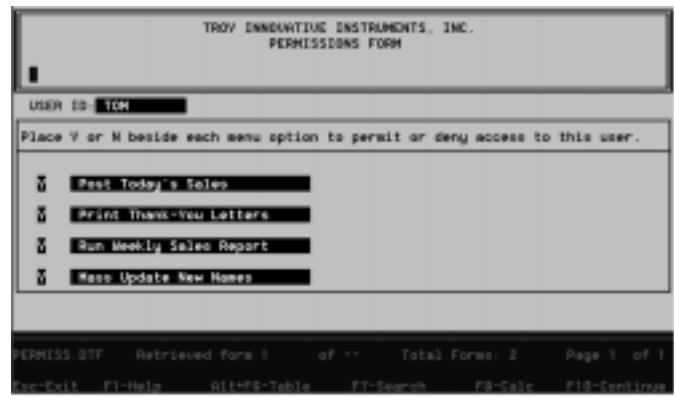
Figure 2. A permissions database that mirrors the menu database, and grants access to the menu selections on a user-by-user basis.
