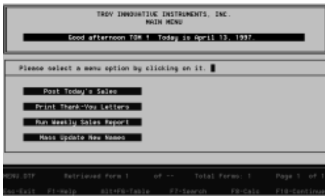
Figure 1. A simple application menu designed in a Q&A database. Behind each selection is a macro that executes when the selection is clicked-on.
