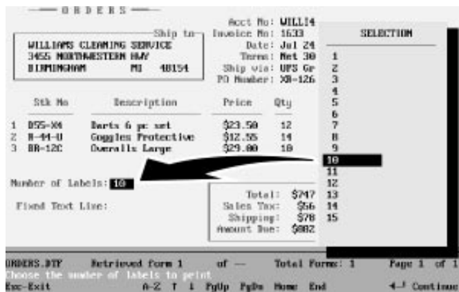
Figure 2. The ORDERS database can be any database from which you might want to print multiple labels for the current record. Here, the Number of Labels field (at the bottom) pops up a selection list for the quantity labels to print. The Fixed Text Line field gives you the option of substituting a fixed text line for the variable text in the current batch of labels.
