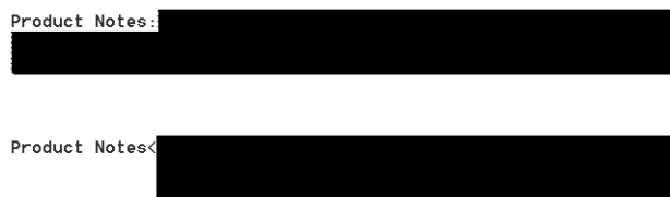
Figure 1 . Using the left angle bracket instead of the colon, you can make a rectangular multiline field.
